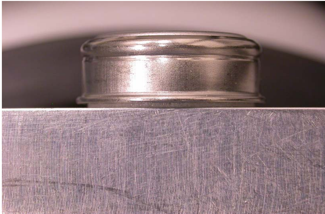
Figure 2.4 - DS1922L attached to the mounting plate with an adhesive pad.
