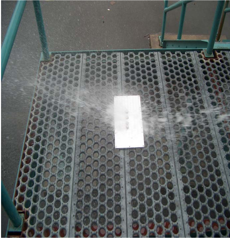
Picture-2. – Water Spray Test Setup (IPX6)
