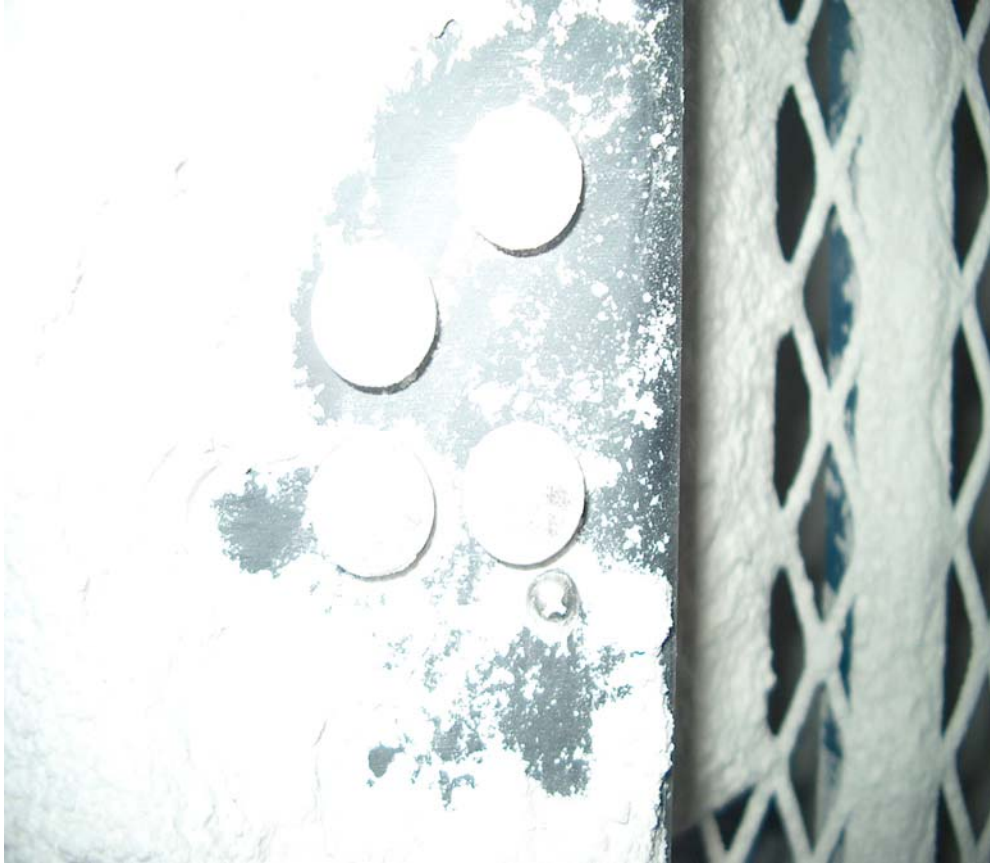
Picture-1. – Dust Test Setup (IP5X)
