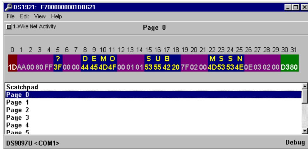
The contents of the memory pages will be color coded to indicate which bytes are length, data and CRC values that conform to the UDP format (see Dallas Semiconductor Application Note 114). The following is a list of the supported color codes in 'Debug' mode:
