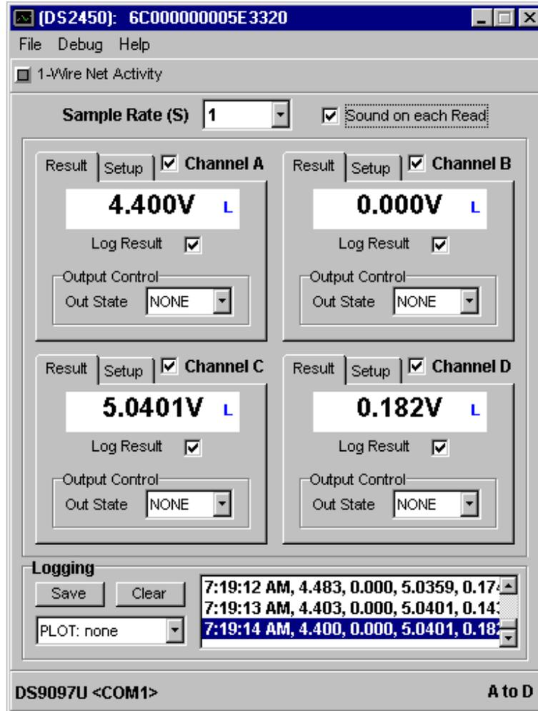
The center box has four smaller boxes representing each of the four A/D channels.
