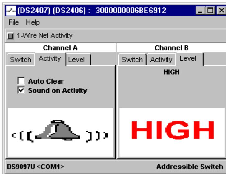
In the **Level** mode, a new sample of the logical level at the I/O channel is taken whenever the device is accessed and displayed as HIGH or LOW in the lower half of the Level tab. In contrast to Activity, which is sensitive to transitions, Level does not catch instances where the voltage level deviates from its quiescent level for a short moment only. In case one needs to see both, one may connect both channels outside of the device and view the activity with one and the level with the other.
