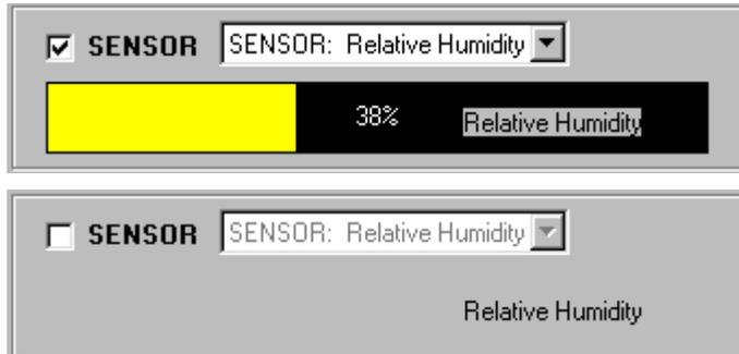
The two images above show the sensor display areas enabled and disabled. If enabled and three other display areas (Temperature, VDD, and VAD) are not, they will automatically be enabled (because calculating sensor data requires Temperature, VDD, and VAD to be enabled). Likewise, if one of the three areas is disabled, the sensor display area will also become disabled.
