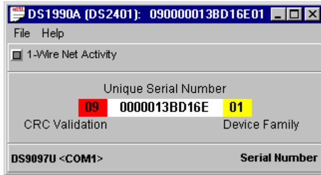
The serial number is displayed in three color coded segments. The left (red) part is the cyclic redundancy check 'CRC' that verifies the integrity of the number. The middle (white) part is the serial number the device was assigned. The right (yellow) part is the device family code. The family code indicates to an application the capabilities of the device. This family code is used by this application to spawn the appropriate viewer.
