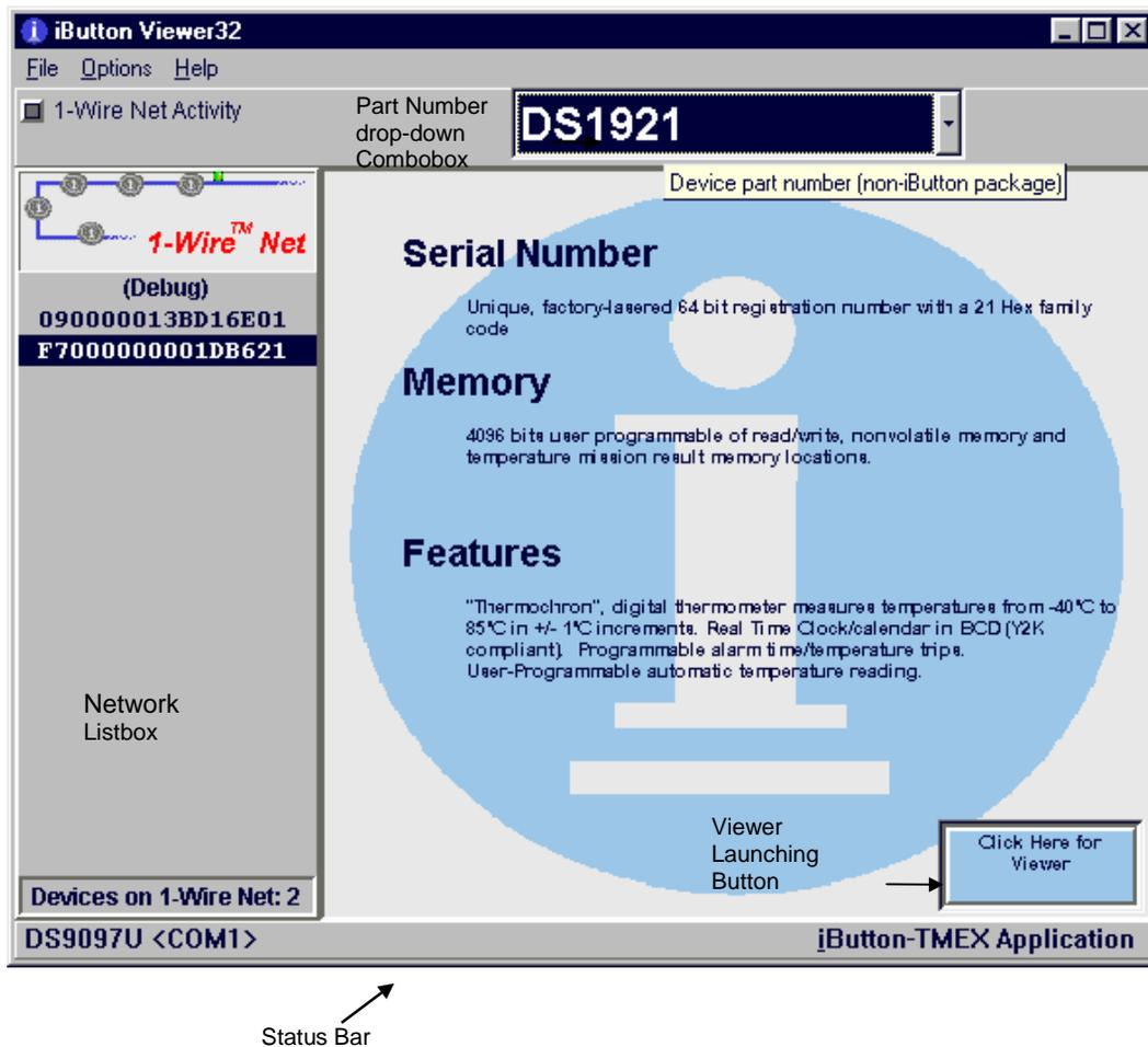
The **Network Listbox** is the primary switchboard of the iButton Viewer. It lists the ROM codes (= network node addresses) of all devices currently connected to the 1-Wire network. The user can scroll through this list with the cursor keys or click on a network node address to select a device. Depending on the number of devices connected, the Network Listbox may have a scroll bar to allow reading all addresses and selecting a device. If no device is connected the Network Listbox will be empty.
