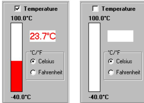
The above images show the temperature display area enabled and disabled. Please note the radio buttons that will allow changing between Celsius and Fahrenheit temperature scales.
