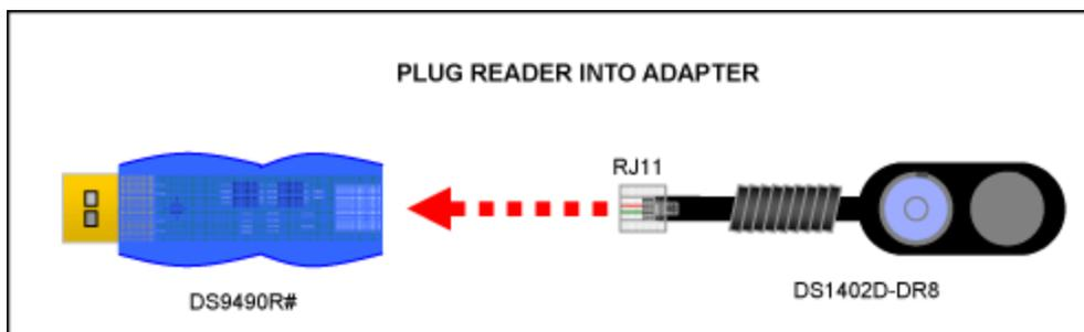
Figure 11. Connect the reader to the adapter.
