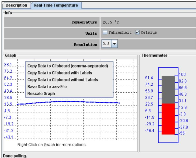
When the Real-Time Temperature tab is active, the Real-Time Temperature viewer:
